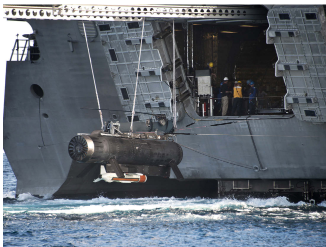
Figure 5 | The Remote Minehunting System (RMS) and an AN/AQS-20 minehunting sonar (attached underneath) are brought aboard the Littoral Combat Ship (LCS) USS Independence. Photo courtesy of Raytheon and the U.S. Navy.
