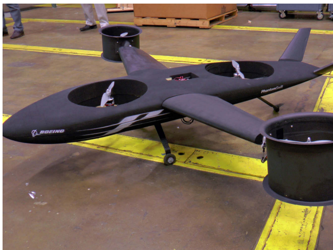
Figure 1 | The Boeing Phantom Swift prototype enables vertical take offs and landings, hovering capabilities, and 400-knot speeds. Photo courtesy of Boeing.
